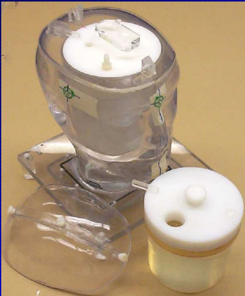
Figure 2: The BANG gel and imaging/dosimetry inserts. Note the PTVs, critical structure and film/TLD provisions in the disassembled imaging insert.
