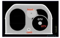
The thorax phantom consists of the following: GTV containing 2 TLD Heart containing 1 TLD
