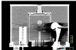
Figure 2 Coronal kVCT slice showing the prosthetic hip location inside the pelvic phantom
