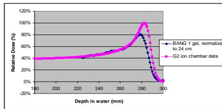
Figure 7. Comparison of the 250 MeV pristine proton depth dose from OCT scans of the BANG<sup>®</sup>1 polymer gel dosimeter and ion chamber measurements.
