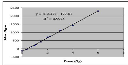
Figure 3. Proton dose response curve of Optical CT signal intensity (attenuation) related to dose for BANG<sup>®</sup>3. Error bars represent one standard deviation of the signal intensity.
