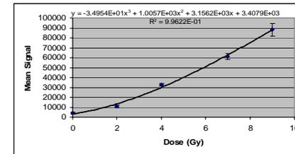
Figure 6. Proton dose response curve of Optical CT signal intensity (attenuation) related to dose for BANG<sup>®</sup>1. Error bars represent one standard deviation of the signal intensity.
