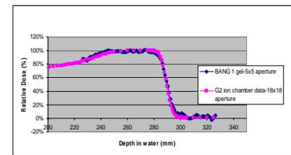
Figure 8. Comparison of the 250 MeV 4 cm modulated proton depth dose from OCT scans of the BANG<sup>®</sup>1 polymer gel dosimeter and ion chamber measurements.
