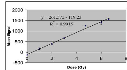
Figure 4. Photon dose response curve of Optical CT signal intensity (attenuation) related to dose for BANG<sup>®</sup>3. Error bars represent one standard deviation of the signal intensity.
