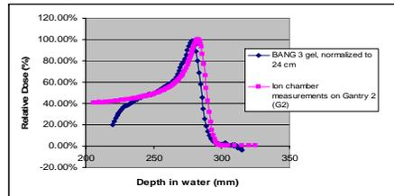
Figure 5. Comparison of the 250 MeV pristine proton depth dose from OCT scans of the BANG<sup>®</sup>3 polymer gel dosimeter and ion chamber measurements.
