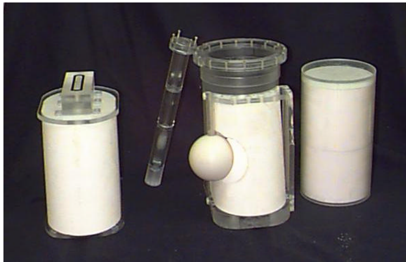
The phantom lungs, spine, heart, and imaging insert.
