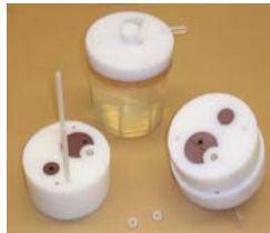
Fig. 2 Polymer gel insert (center) with the disassembled planning insert. The primary and secondary target volumes are the brown structures. The OAR is the small Lucite cylinder partially encompassed by the primary target volume. Note the acrylic external registration key on both the gel and planning inserts.
