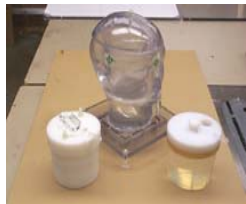
Fig. 1 Images of the currently used IMRT head and neck phantom (above) and the redesigned version that facilitates polymer gel dosimetry (below).
