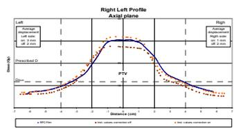
Fig 5: Dose profile comparison on the transverse axis. The displacement between film values and TPS values is presented for both situations (correction on and off).
