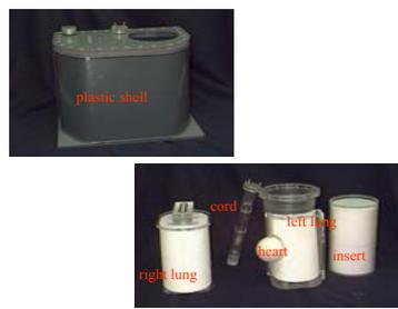
Fig 1: Thorax phantom: plastic shell and internal structures
