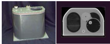
Fig. 1. Anthropomorphic phantom and axial CT image.
