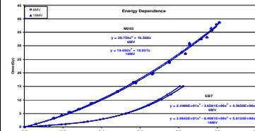
Fig.3: EBT and MD55 dose response at 6 and 18 MV photon beam.
