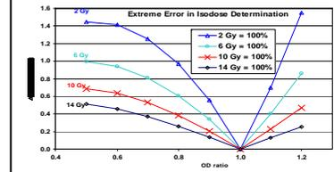
Fig.5: Extreme error in isodose determination for EBT film irradiated with 6MV photon beam. Analysis done for a specific batch.
