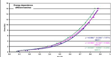
Fig.4: Dose vs. OD for three different batches of EBT film.
