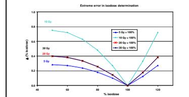
Fig.6: Extreme error in isodose determination for MD55 film irradiated with 6MV photon beam. Analysis done for a specific batch.
