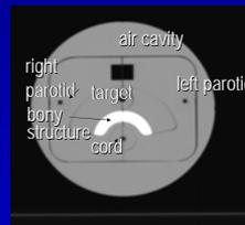
Figure 1. Axial CT image of the phantom
