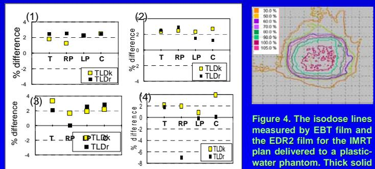
Figure 3. % differences of (1) case 1, (2) case 2, (3) case 3, and (4) case 4. Data were normalized to IC measurements. TLDk: KFDA data, TLDr: RPC data. T: target, RP: right parotid, LP: left parotid, C: spiral cord.
