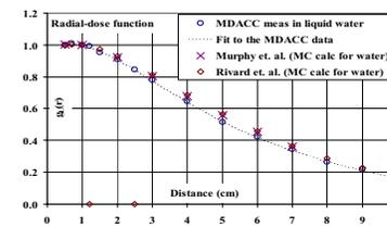
Fig. 4: Radial dose function measured in water.
